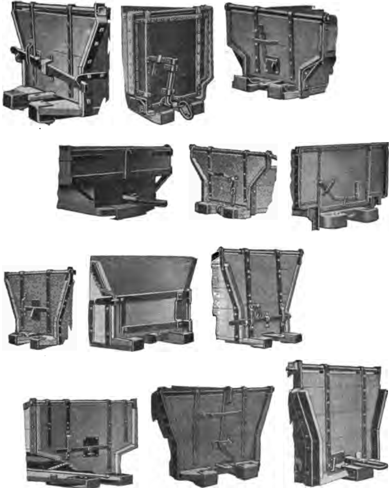
Fig. 2. Latches Used on End Gates.
